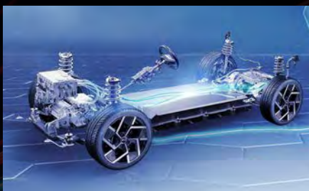
Safety - E-Platform 3.0 With The Cell-to-Body (CTB) Structure
